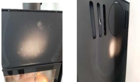
Picture 10. Examples of housing discoloration caused by overheating.
