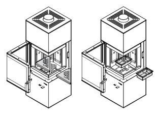
Lift the ash-pan holding the handle and carefully remove it after removal of second part of grate. It is recommended to remove dust from ash-pan chamber and furnace.
