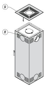
Break off the given plug from the body and then fix entirety by tightening screws on top and bottom of the stove. 9. Finally, install top plate.
