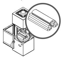
Picture 9. Method of fuel arrangement during firing up.
