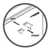
Picture 8. Adjustment of air inflow in DEFRO HOME QUADROOM stove: controller with I symbol control flow of primary air, while controller II controls the secondary air.
