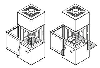
Remove both parts of the grate after opening of the doors. Fist, lift and remove one of the halves.
