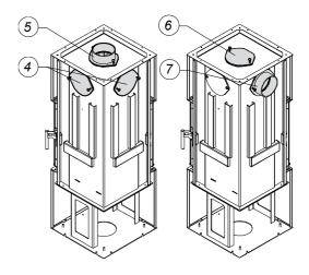
Remove selected plug. 5. Remove screws fixing socket of the flue and hold the second deflector to which the flue is fixed. 6. Tighten plug on top side of the stove to a structure of upper deflector. 7. Remove socket of flue.
