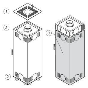
Lift plate on top wall of the stove. 2. Remove screws fixing
