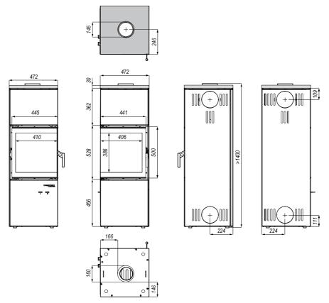
Picture 4 Dimensions of DEFRO HOME QUADROOM dry stove in STONE version (in mm).
