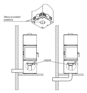
Picture 6. Connection of the dry stove DEFRO HOME QUADROOM to external air inlet.
